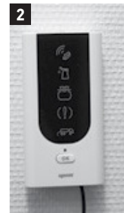
2 Plug the Info panel into an electrical outlet through the included AC adapter and mount it in a wall mount.
