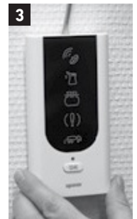
3 To detach the Info panel from the wall bracket, press on the top, for instance, with a screwdriver tip.
