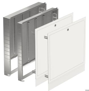
The range of Uponor Vario cabinets IW includes six different cabinet widths for universal use, even in large projects. These cabinets are available in two wall installation depths: IW 110 and IW 80. They are made of rigid galvanised sheet steel construction with all visible components white powder-coated (RAL 9016).
