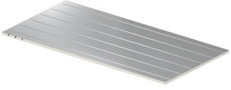
The Uponor Siccus Mini panel is an XPS panel grade 400kpa with dimensions 1200 x 600 x 15 mm and can be installed on top of the existing floor. The prefabricated panel is integrated with pipe grooves with a fixed pipe spacing of 100 mm.
