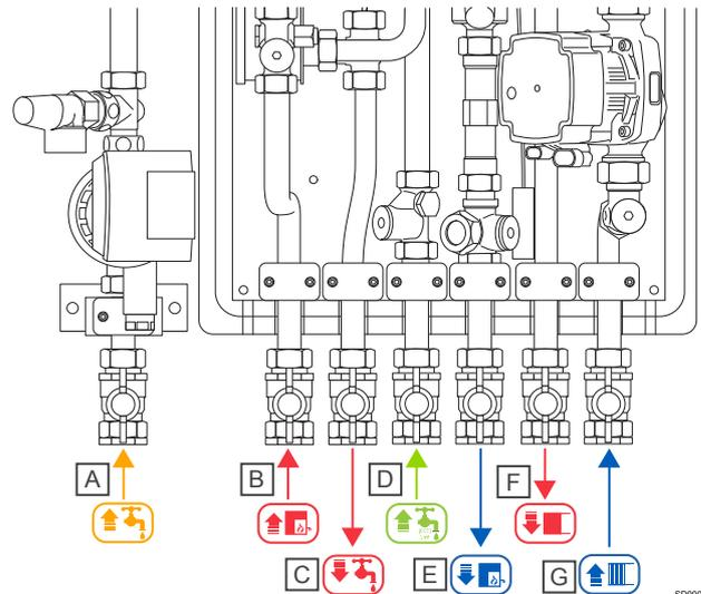
Ball valves B, D and E must be closed in the event of a malfunction.
