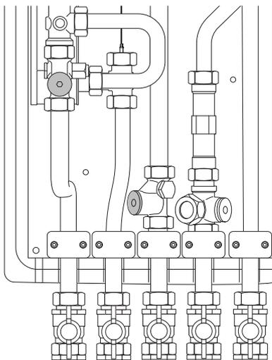
The strainer collects dirt and its filter can be removed for inspection and cleaning.
