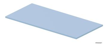
The Uponor Multi insulation panel is a XPS 400 thermal insulation panel with dimensions 1250 x 600 x 20 mm. The panel is ideal for use in front of a manifold, allowing for easier installation of heating pipes.
