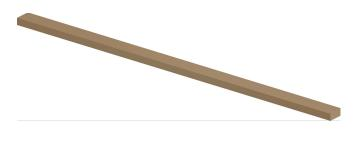
The Uponor Siccus 16 edge support is a MDF strip with dimensions  $1000 \times 45 \times 19$  mm and is ideal for installing on the wall sides and in doorways. The edge support is only used for tiles or natural stone installations, not for direct parquet or laminate installations.
