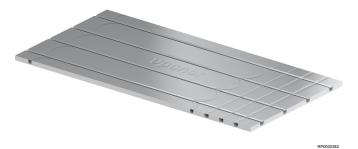
The Uponor Siccus 16 panel is an EPS400 panel grade 400kpa with dimensions  $1200 \times 600 \times 20$  mm and can be installed on top of the existing floor. The prefabricated panel is integrated with pipe grooves with a fixed pipe spacing of 150 mm.
