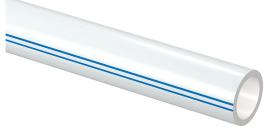
The Uponor Comfort Pipe PLUS is a highly flexible PE-Xa pipe with 5 layers available in the dimension 16 x 2,0 mm.
