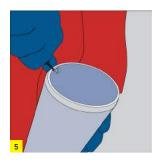
Remove the burrs on the external edges with a knife or scraper.
