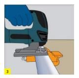
Cut in 90° angle by using a coping saw or a proper cutter.
