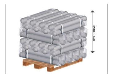
Method of storage should not cause any outflow and should not damage the pipes. As long as they are stored properly, no permanent deformations or damages will occur on the pipes and fittings. Pipes should not be stacked above 1,5 m. Pipes should be safe against sliding.
