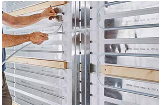
Uponor Siccus heat conducting lamellas – stable aluminium lamellas with omega groove for optimal heat transfer to the system pipe 2-fold pre-punching for simple shortening without tools of the lamella size 120 x 1180 mm.
