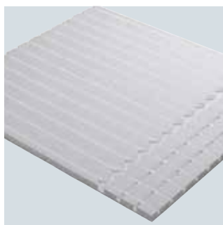
Uponor Siccus laying plate – laying plate made of EPS with pipe routing channels for holding the Uponor Siccus heat conducting lamellas. Laying spacing 15 / 22.5 / 30 cm.
