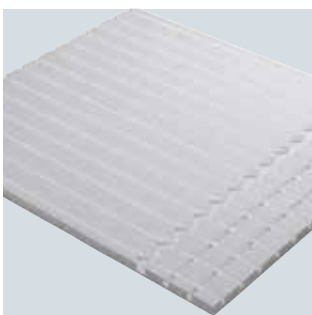
Uponor Siccus plate – laying plate made of EPS with pipe routing channels for holding the Uponor Siccus heat conducting lamellas. Laying spacing 15 / 22.5 / 30 cm.
