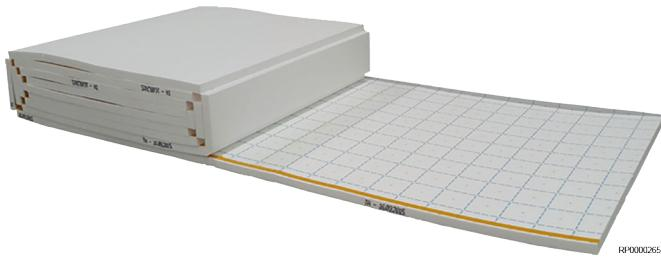
The Uponor Klett panel roll is an EPS DES panel with added graphite and ideal for increased heat insulation and low-height floorconstructions. It is available in versions 25-2, 30-2, 30-3, 35-3 and integrated with thermal and impact sound insulation as per DIN EN 13163.
