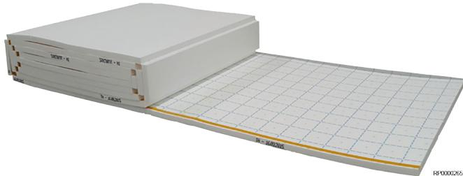
The Uponor Klett panel roll is an EPS DES panel with added graphite and ideal for increased heat insulation and low-height floor constructions. It is available in versions 25-2 and 40-2 and integrated with thermal and impact sound insulation as per DIN EN 13163.
