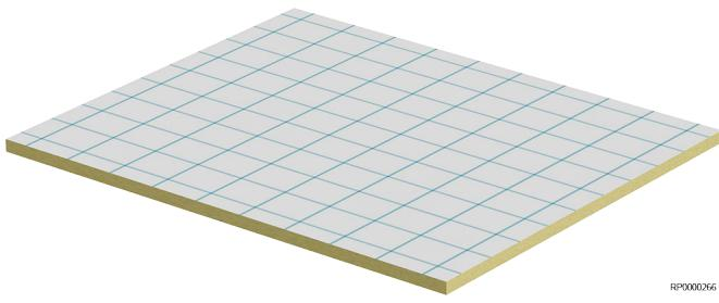
The Uponor Klett Silent is a mineral fibre insulation panel and is ideal for optimised impact sound insulation and low-height floor constructions. Reducing the pipe coverage to 30 mm is possible using Knauf liquid screed FE 80 ECO. With the test results, the system has proven to be low-emission.
