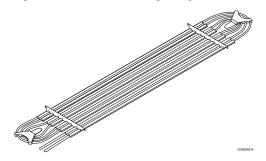
The panels consist of Uponor Comfort pipe 9.9 mm, pre-assembled with galvanized steel heat spreaders in different length. The joint spreaders enable fast snap mounting within the CD profiles of the ceiling substructure. Due to straight and even steel lamella with some flexibility in fixation, the installed panels will have full surface contact to gypsum cladding for best thermal performance.
