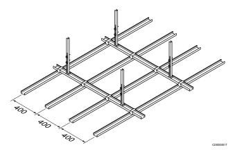
The Uponor Thermatop S heating and cooling panels are installed suspended within regular substructures (on site), between the CD 50 mm or CD 60 mm profiles of the ceiling structure. The planning/mounting guidelines of the ceiling manufacturer are to keep.
