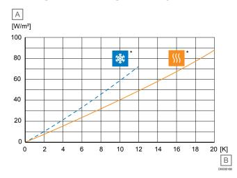
\*) Nominal heating and cooling capacity of Uponor Thermatop S with 10 mm gypsum board (0,25 W/mK)
