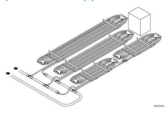
Due to wide portfolio to connect Thermatop S panels to a complete thermal active ceiling, Uponor recommends the installation with Uponor Comfort Pipe PLUS or Uponor Uni Pipe in our design services to enable full system.
