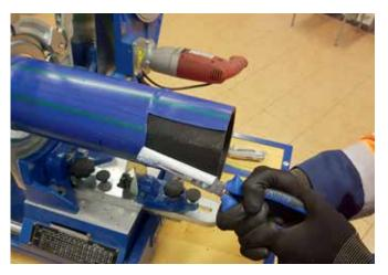
2. Grip the edge of the layer with pliers and roll the part that is to be removed around the pliers.
