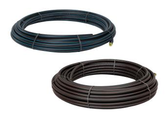
PE80 pressure pipes are produced of polyethylene, a safe and secure material for handling of potable- or sewer water. All dimensions are available in coils, making it possible to do long installations without any connections. PE80 is a very flexible plastic material, it is easy to work with and change of direction can be done without elbows. Due to this flexibility, the pipe is not sensitive to settlements and movements in the surrounding soil.
