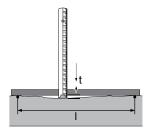
For parquet/ laminate flooring, wooden beam construction with a max. deflection of I/500 is permitted.
