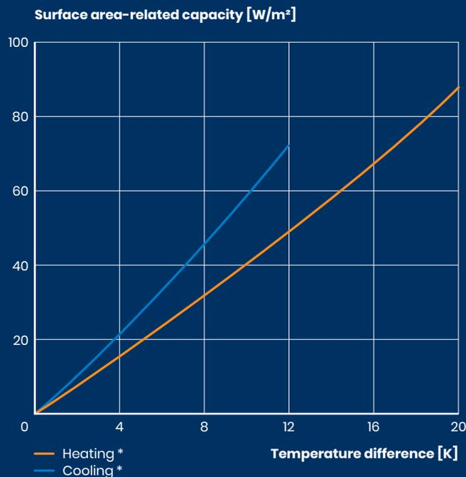
\* Heating and cooling capacity of Uponor Thermatop S with 10 mm gypsum board (0,25W/mK)
