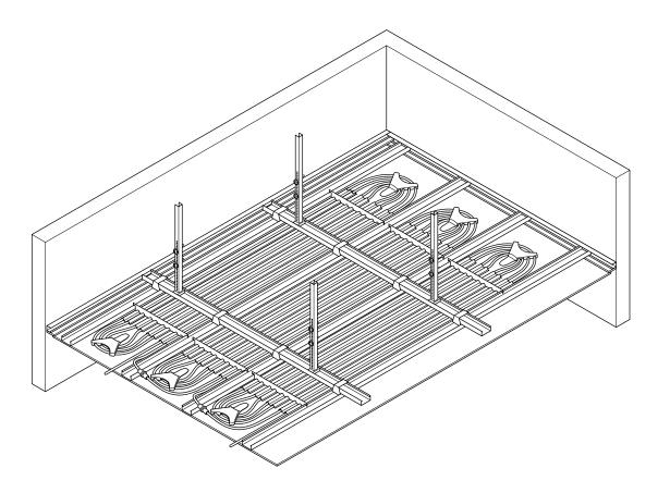
Uponor Thermatop S is a radiant heating and cooling ceiling system that operates primarily according to the radiation principle, working inaudible and invisible inside seamless gypsum ceilings.
