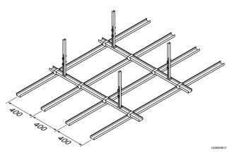
The Uponor Thermatop S heating and cooling panels are installed suspended within regular substructures (on site), between the CD 50 mm or CD 60 mm profiles of the ceiling structure. The planning/ mounting guidelines of the ceiling manufacturer are to keep.
