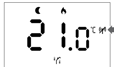
Figure 1. Example from a heating system operating in eco mode without demand, in control mode RO
