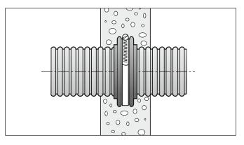
Mounting the wall through sealing NPW
