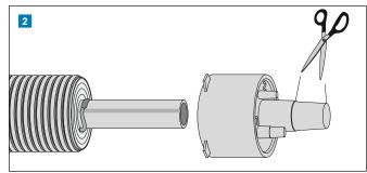
Carry out the termination using the installation set Supra PLUS 2 (separate installation instructions for the electrician).
