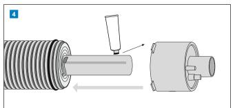
Pull the end cap on top of the pipe element using lubricant.
