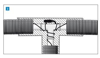
Join the ends of the heating cables with Supra PLUS 2 installation set equipment and wrap the heating cables on the branch with heatproof tape (electrician).
