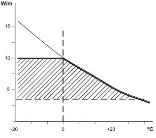
The heating cable supplies full power in ice, cold water or in frozen pipeline. The ruled area in the image shows the input power W/m depending on the outdoor temperature when the heating cable is on continuously.
