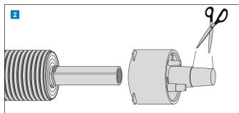
Carry out the termination using the installation set Supra PLUS 1 (separate installation instructions for the electrician).
