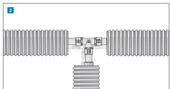
Join the service pipes with couplings (not included in the set). If required, the end caps are installed in place before joining the service pipes. Be careful not to damage the heating cable. Note the required shrinks for insulating the branch tee before installing the fasteners. Use the insulation that was peeled off as an additional insulation for the joint.
