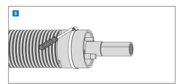
Place the clamping ring above the seal on the end cap and tighten.
