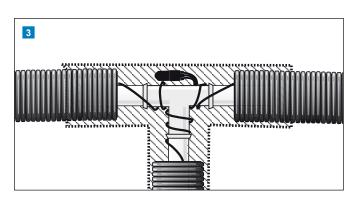
Join the ends of the heating cables with Supra Standard 2 installation set equipment and wrap the heating cables on the branch with heatproof tape (electrician).
