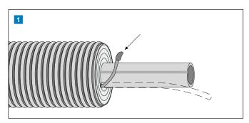
Peel off the casing pipe and remove the insulation taking into account the length of the end cap. Reserve 0.5 m of cable for the electrician. Cut the service pipe at the required length. Do not damage the cable or the service pipe. Clean thoroughly (including the casing pipe).
