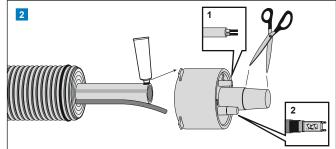
Install the sensor. Pull the end cap on top of the pipe using lubricant.
