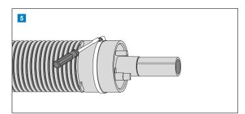
Place the seal in its place in the 2nd or 3rd groove. Cut the output for the service pipe of the end cap at the correct dimension.
