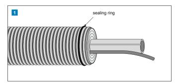
Peel off the casing pipe and remove the insulation taking into account the length of the end cap. Reserve 0.5 m of cable for the electrician. Cut the service pipe at the required length. Do not damage the cable or the service pipe. Clean thoroughly (including the casing pipe).
