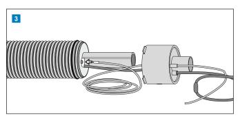
Carry out the extension using the heating cable - supply cable installation set Supra PLUS 1 (separate installation instructions for the electrician).
