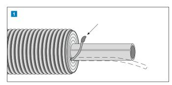
Peel off the casing pipe and remove the insulation taking into account the length of the end cap. Reserve 0.5 metres of cable for the electrician. Cut the service pipe tube at the required length. Do not damage the cable or the flow pipe. Clean thoroughly (including the casing pipe).
