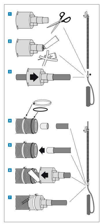
The installation of Supra Mantle is easiest when the water pipe is installed before any connectors are connected to the water pipe. The jacket is slid on the water pipe in the correct place and then the jacket containing the water pipe is installed in the correct location.
