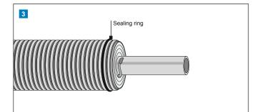
Place the seal in its place in the 2nd or 3rd groove. Cut the output for the service pipe of the end cap at the correct dimension.
