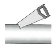
2. Make a chamfer to the pipe end.
