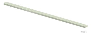
Uponor Siccus Mini edge support is a synthetic strip with dimensions  $1000 \times 45 \times 15$  mm and is ideal for installing on the wall sides and in doorways. The edge support is only used for tiles or natural stone installations, not for direct parquet or laminate installations.
