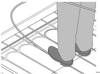
4. Connecting pipes to the manifold
