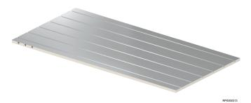
The Uponor Siccus Mini panel is an XPS panel grade 400kpa with dimensions  $1200 \times 600 \times 15$  mm and can be installed on top of the existing floor. The prefabricated panel is integrated with pipe grooves with a fixed pipe spacing of 100 mm.
