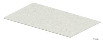
The Uponor Siccus Mini tile-backer panel is a synthetic panel with dimensions  $1000 \times 600 \times 6$  mm and it must be installed on top of the existing panel as a load distribution layer for tiles and natural stone.
