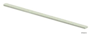
Uponor Siccus Mini edging strip is a synthetic strip with dimensions  $1000 \times 45 \times 15$  mm and is ideal for installing on the wall sides and in doorways. The strip is only used for tiles or natural stone installations, not for direct parquet or laminate installations.
