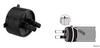
Uponor Ecoflex rubber end caps protect pipe-end insulation from moisture and potential damage to ensure optimal system operation. It is assembled by sliding over the pipe ends and securely affixed using a clamping ring.
