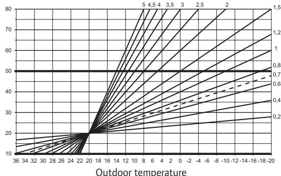
The choice of curve depends on a combination of different factors, such as how well insulated the house is, geographical location, type of heating/cooling system etc.
