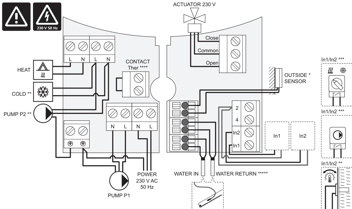
\*) The outdoor temperature sensor can be connected to either the controller or to a thermostat (requires antenna A-155).
