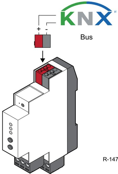
To connect the KNX gateway module to the Base PRO controller:
