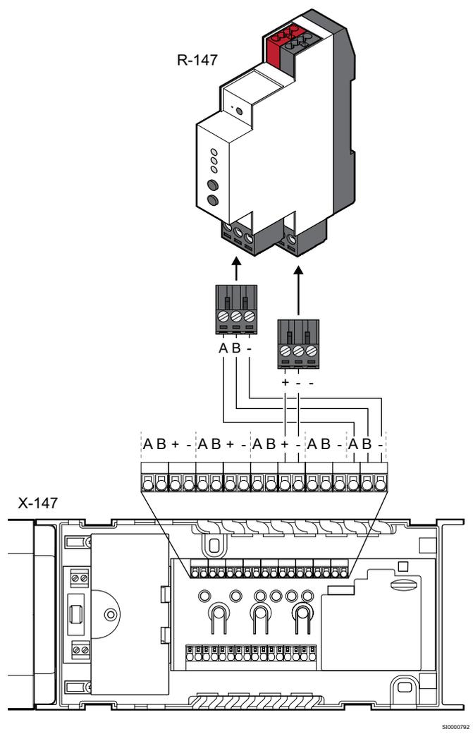
To connect the KNX gateway module to the Base PRO controller:
