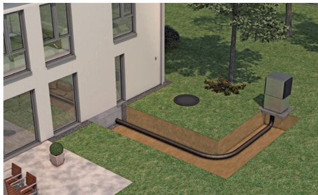
Connection of Uponor Ecoflex Thermo Twin HP between an external heat pump and residential building
