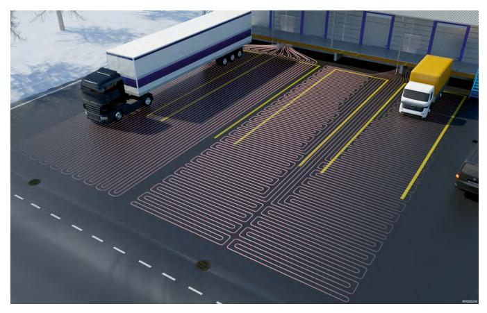
This illustration shows an example of a truck loading area with an Uponor Meltaway system design. There are four equal sized (160 m<sup>2</sup>) melting areas designed using two separate manifolds.
