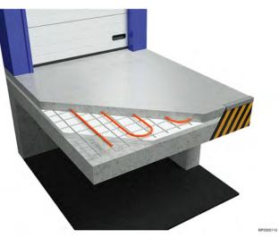
The need for insulation is normally low because of the high temperature difference between the heated surface outdoors and the ground. But when designing deck structures, like loading areas or bridges, the structure will also cool from underneath. In these cases it is recommended to use insulation in the structure to prevent heat loss downwards.
