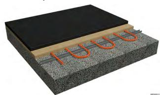
The image shows the basic installation of an asphalted structure with low wear. Mainly used for parking areas and truck loading areas with low traffic.
